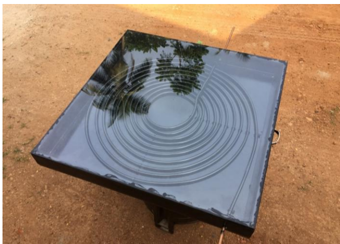
Fig.4 Solar water heater
