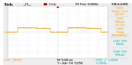
Fig.20. Voltage across upper and lower diodes
