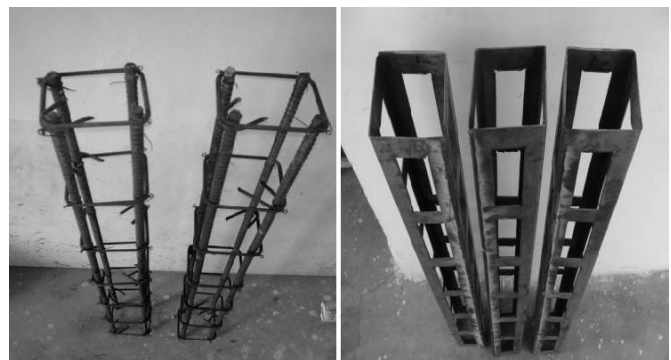
Figure 1. Rebar reinforcement and Prefabricated Cage System
