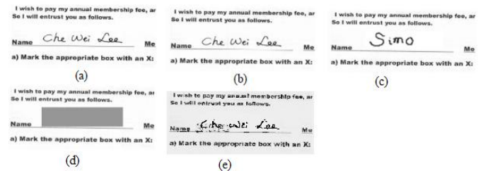
Fig. 4. Authentication result of a TIFF document image of a signed paper attacked by superimposing a white rectangular shape on the signature. (a) Original cover image. (b) A stego-image with embedded data. (c) Tampered image yielded by the superimposing operation. (d) Result with tampered blocks detected and marked as gray. (e) Data repair result.
