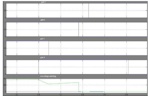
Fig.14. Zero voltage switching in mode 6.
