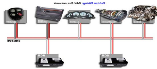
Fig 2: A simple CAN bus connection
